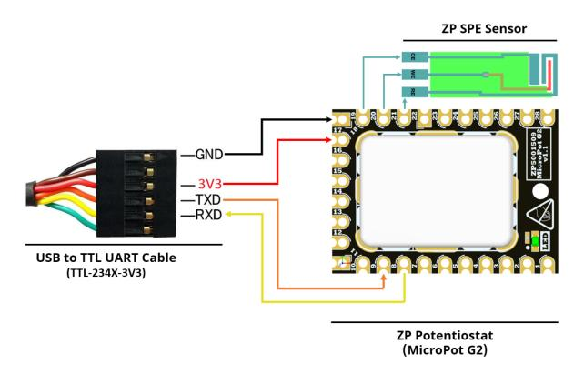
Figure 1. Basic MicroPot G2 Test Setup
