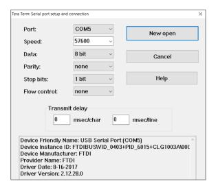
Figure 3. TeraTerm setting window for COM port connection
