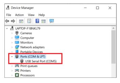
Figure 2. Device Manager COM Port enumeration
