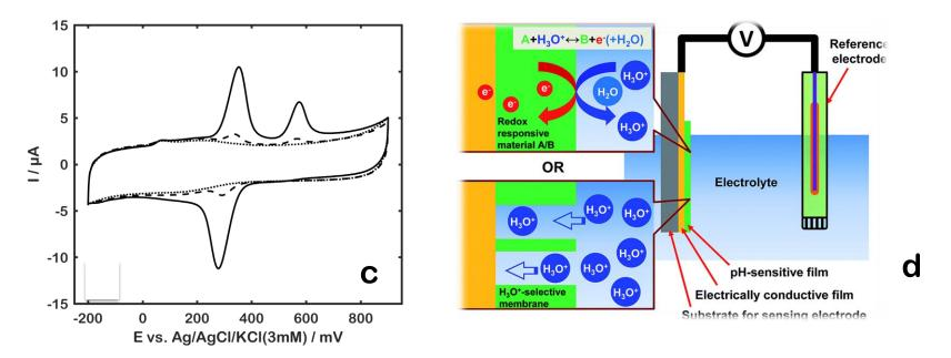
**Figure 2.** (a) Amperometric detection of glucose (b) voltametric detection of electrochemically active species (c) Baseline corrected voltammogram (—) obtained through subtracting the baseline (…) from the raw signal (--). (d) Potentiometric of ions including, sodium, potassium and pH.
