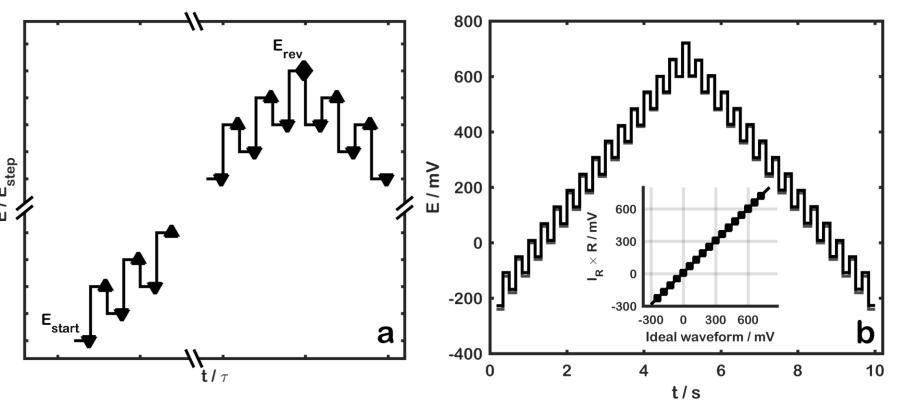
**Figure 5.** (a) Squarewave voltage waveform. Down-pointing and uppointing triangles marks where the reverse and forward current is sampled, respectively. (b) Simulated waveform (gray) and waveform from sensor platform (black) obtained by multiplying the squarewave current  $I_R$ , with the load resistance, R. The inset shows the relationship between actual and simulated waveforms.
