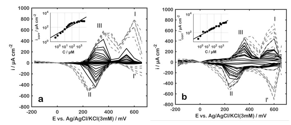
**Figure 6.** Baseline corrected coarse cyclic squarewave voltammograms (second scan) from **(a)** commercially sourced electrodes and potentiostat, and **(b)** sensor platform with integrated electrodes and electronics. The dotted lines (--) represent the signals which satisfies  $I \ge I_{III}$ . The insets show the corresponding calibration curves from Eq. (1).
