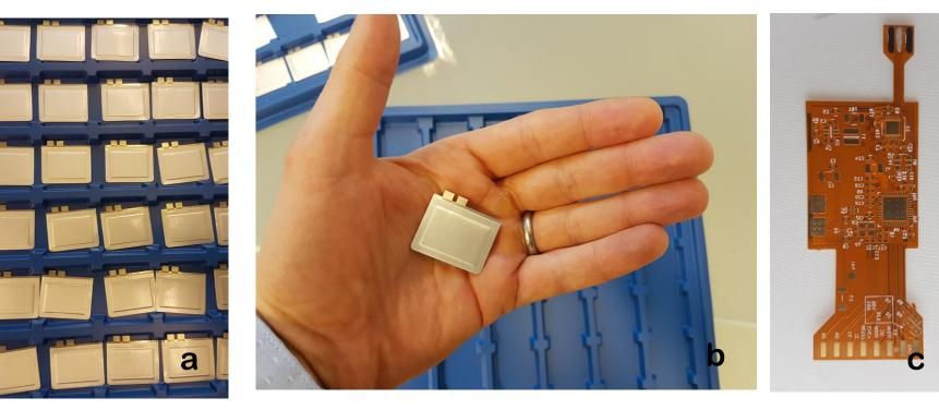
**Figure 3.** (a) The think lithium polymer battery (b) The think lithium polymer battery (c) The biosensor and electronics are mounted on the same flex pcb.
