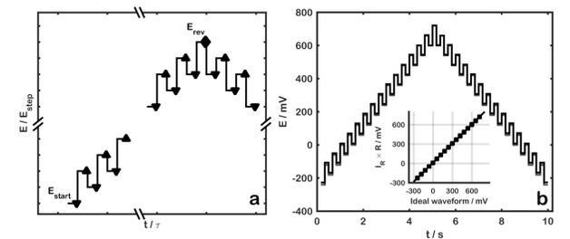
**Figure 5.** (a) Squarewave voltage waveform. Down-pointing and up-pointing triangles mark where the reverse and forward current is sampled, respectively. (b) Simulated waveform (gray) and waveform from sensor platform (black) obtained by multiplying the squarewave current  $I_R$  with the load resistance, R. The inset shows the relationship between actual and simulated waveforms.
