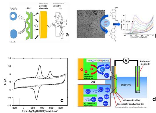
**Figure 2.** (a) Amperometric detection of glucose (b) voltammetric detection of electrochemically active species (c) Baseline corrected voltammogram (—) obtained through subtracting the baseline (---) from the raw signal (---). (d) Potentiometric of ions including, sodium, potassium and pH.
